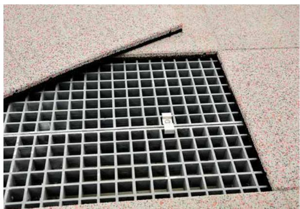
The approximately 11 mm thick, highly resilient EPDM wear layer is resistant to the usual stresses as well as steel runners, sticks and ski-shoes, and moreover it has excellent non-fade properties. It is pleasant to walk on thanks to the PUR-bonded rubber fibres of the approximately 19 mm thick soft base layer. The colour scheme of the slabs, which are 30mm thick in total, was designed in accordance with client's wishes and was matched to the floor materials on the other levels.
